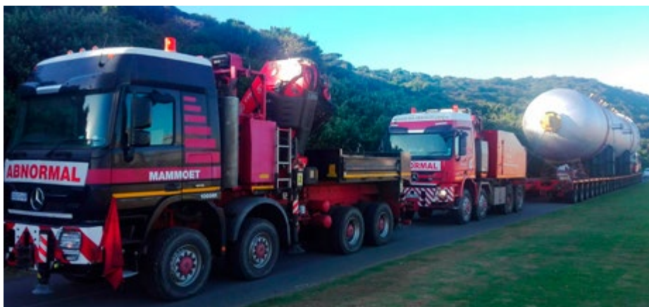
280-ton reactor being moved from Durban port, another Oil and Gas project.
